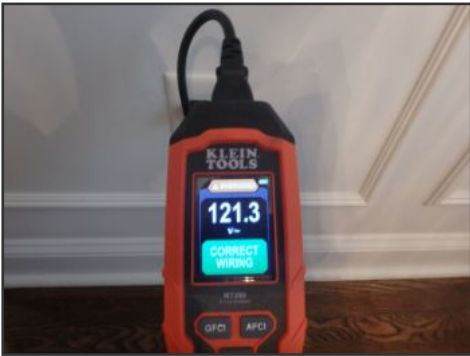
example receptacle testing
