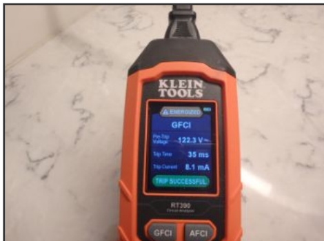
example GFCI testing
